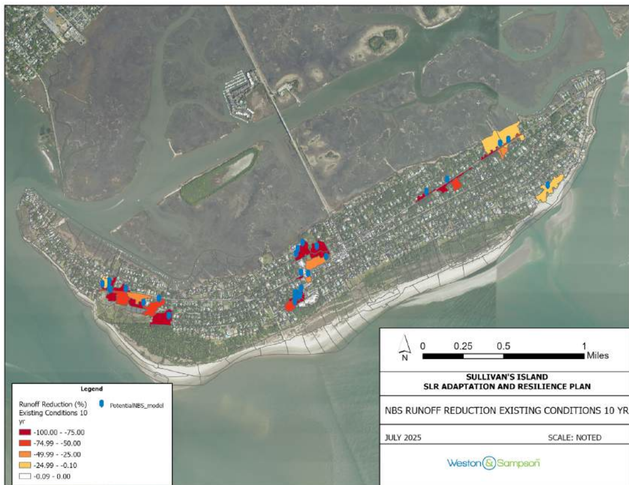
Figure 64: Percentage of Runoff Reduction from NBS for Existing Current Conditions 10 yr Rainfall
