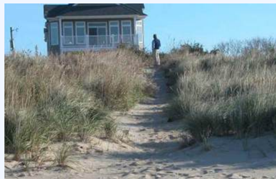
Figure 46: An example of an effective access path through dunes where no dune walkover is needed.
