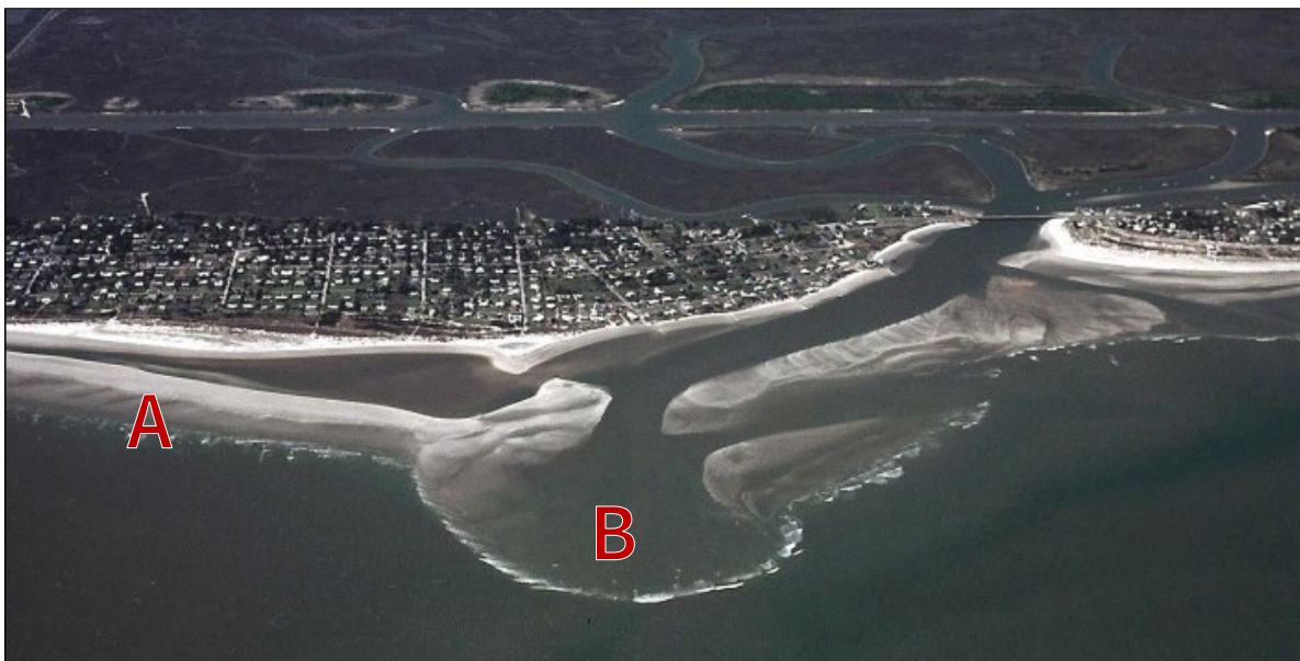
FIGURE 1.6. Oblique aerial photograph at low tide showing the deflection of Breach Inlet around shoals extending from Isle of Palms (right side of photo). Breaks in the shoals (B) allow the channel to shift, freeing sand further west (A) to move onshore and accrete along Sullivan's Island. [Photo circa 2005 by TW Kana]
