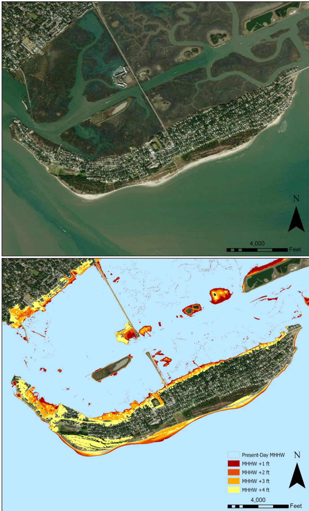
FIGURE 4.5a,b. Sea level inundation models around the Sullivan's Island generated using data from NOAA ( https://coast.noaa.gov/digitalcoast/tools/slr.html ). Shades of yellow, orange, red, and maroon are used to signify SLR of 1, 2, 3, and 4 ft above present-day MHHW.
