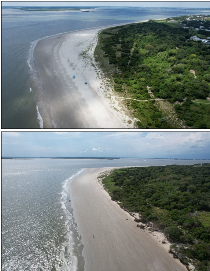
FIGURE 3.10. Aerial imagery indicating the extent of upland encroachment by the MHW line between August 2023 (upper) and September 2024 (lower).
