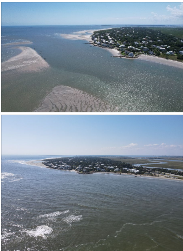
FIGURE 3.14. Beach volume and width changes around Breach Inlet are strongly impacted by shifts in the position of the primary inlet channel seen here. Aerial imagery between August 2023 (upper) and September 2024 (lower) documents the attachment of a shoal just west of Reach 4, and the static nature of the beach-upland boundary along the reach due to the presence of armor stone revetments. A USACE beneficial use project scheduled for 2024–2025 is expected to place more than 200,000 cy below MLW along the reach. Coupled with a Town-sponsored effort to recycle some of that sand into the dune, the beach condition of Reach 4 should improve between September 2024 and the 2025 annual survey.
