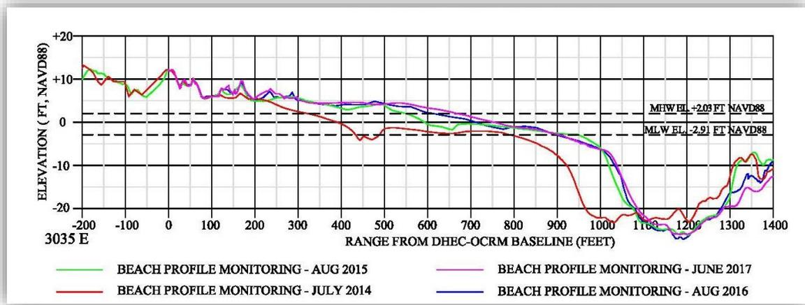
Figure 13. Beach profile monitoring data from 2014-2017 in cross-section view at Monument 3035.
