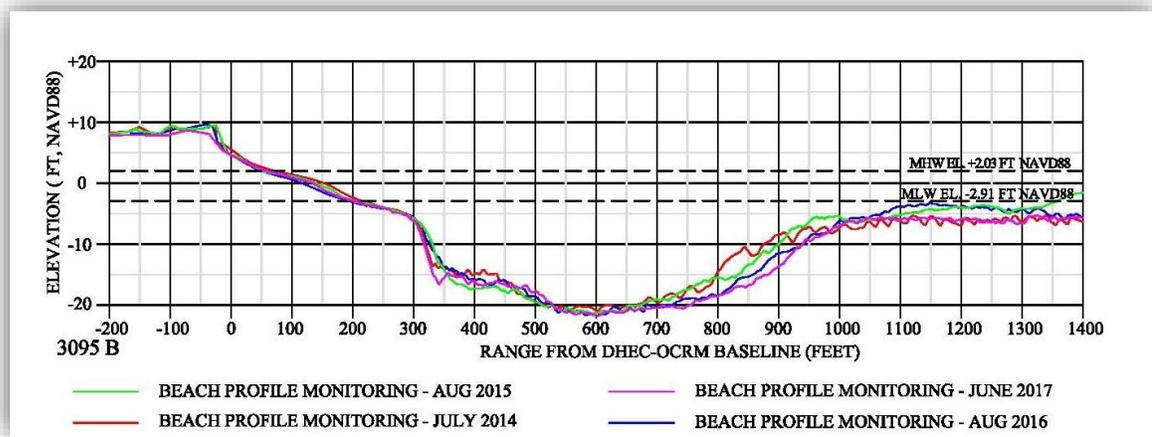
Figure 37. Beach profile monitoring data from 2014-2017 in cross-section view at Monument 3095.
