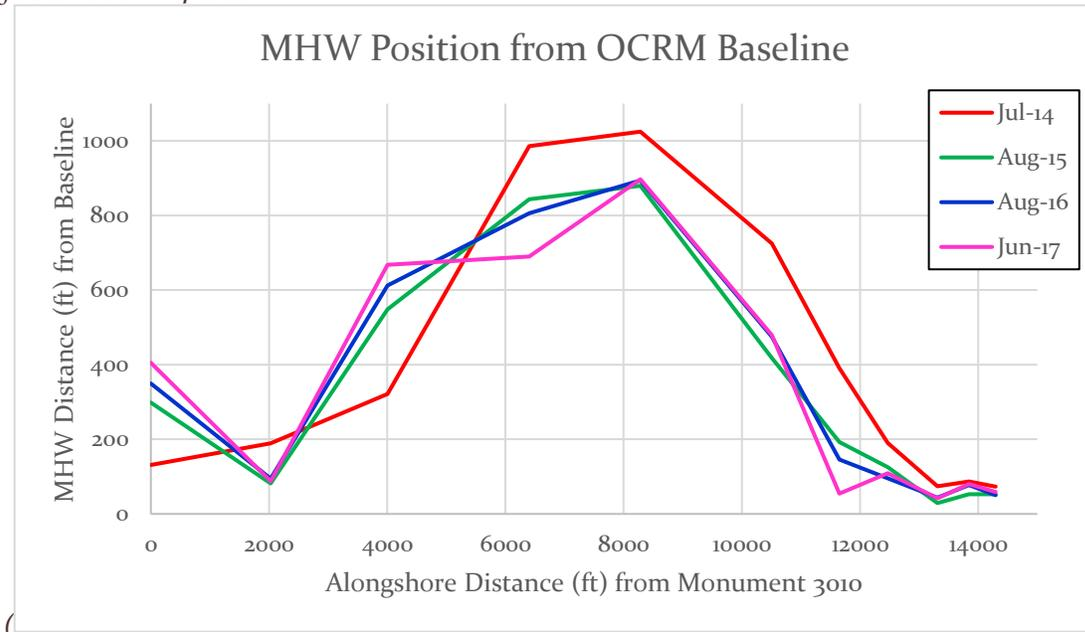
Figure 5). This dramatic shoreline retreat has stopped and shoreline positions have stabilized at most of the monuments in this section with two previously mentioned exceptions.
