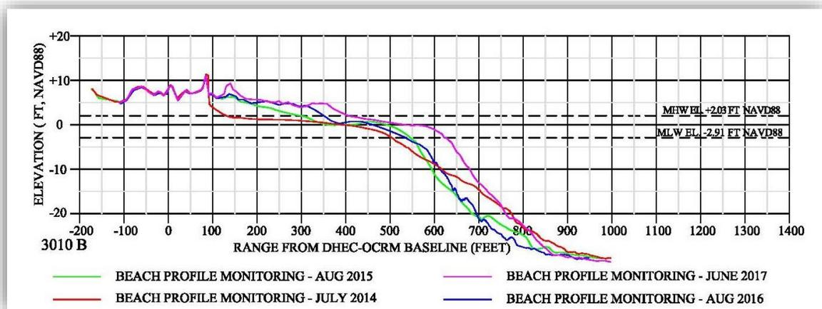
Figure 7. Beach profile monitoring data from 2014-2017 in cross-section view at Monument 3010.
