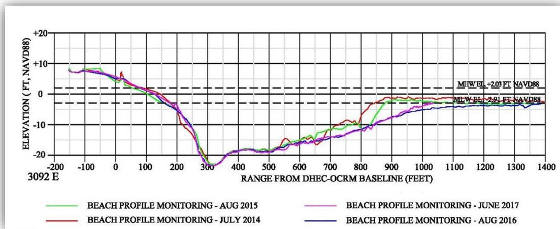
Figure 34. Beach profile monitoring data from 2014-2017 in cross-section view at Monument 3092.
