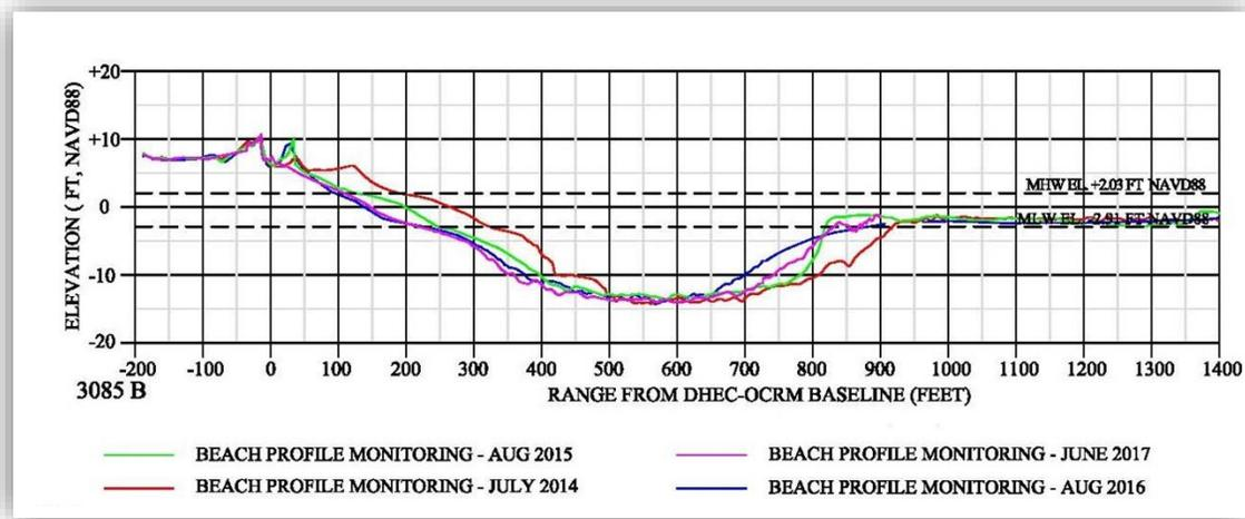
Figure 28. Beach profile monitoring data from 2014-2017 in cross-section view at Monument 3085.
