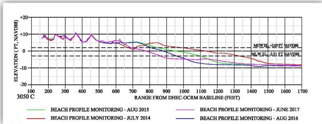
Figure 16. Beach profile monitoring data from 2014-2017 in cross-section view at Monument 3050.
