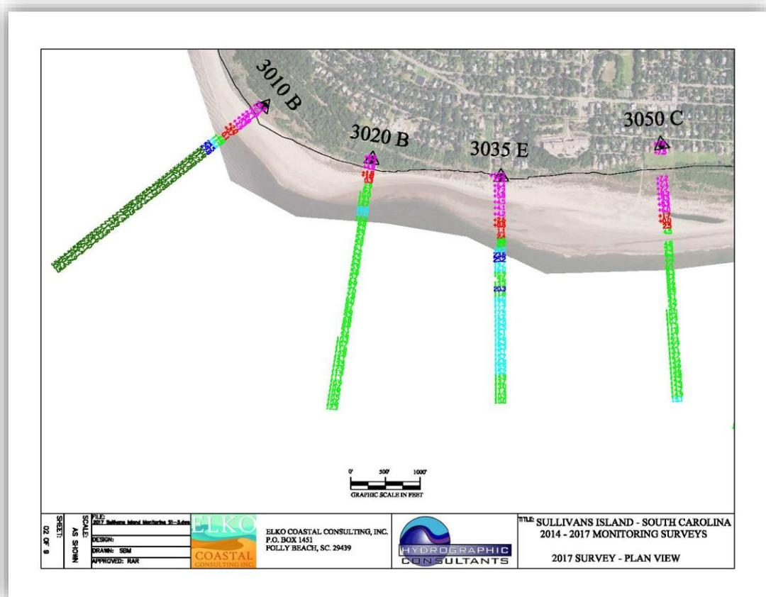
Figure 3. Topographic and bathymetric 2017 survey data illustrating the measured elevation along each line for the southwest end of Sullivan's Island.
