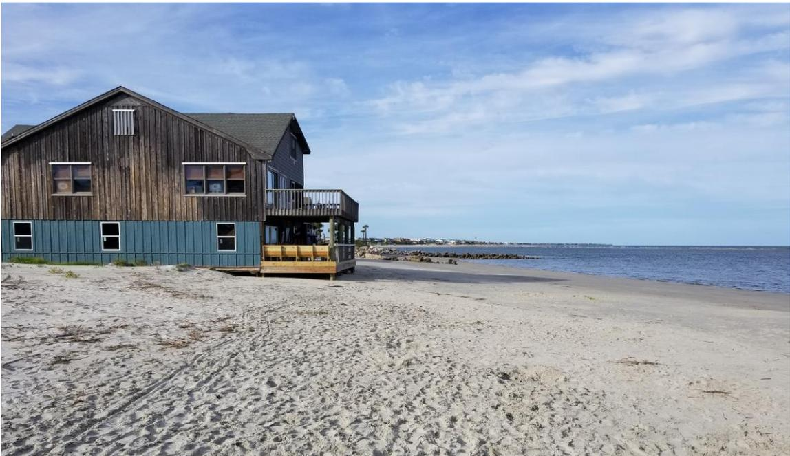
*Figure 29. Ground photo taken at Monument 3085 looking northwest on August 4, 2016 (top) and June 12, 2017 (bottom). Notice the profile deflation under the deck in 2017.*
