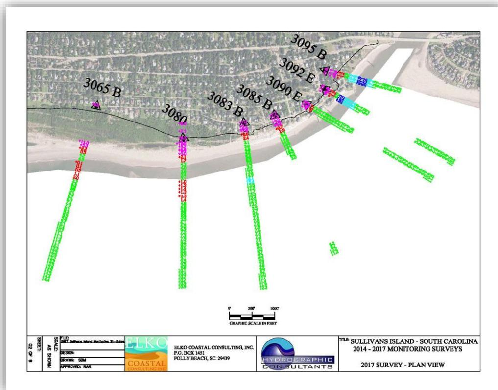
Figure 4. Topographic and bathymetric 2017 survey data illustrating the measured elevation along each line for the northeast end of Sullivan's Island.
