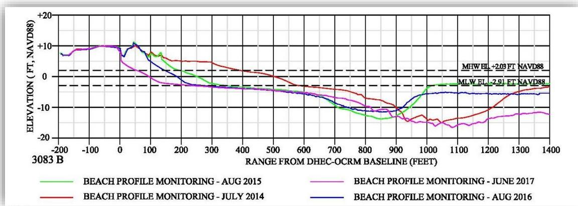
Figure 25. Beach profile monitoring data from 2014-2017 in cross-section view at Monument 3083.
