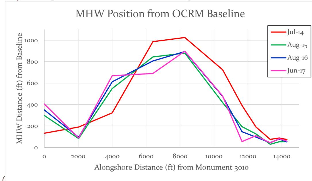
Figure 5) because it illustrates both the change in shoreline position from year to year, as well as the distance between the shoreline and baseline – an indicator of the level of storm damage protection provided by the beach/dune system at each monument.
