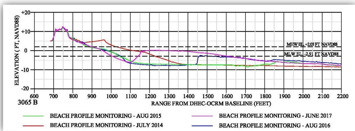
Figure 19. Beach profile monitoring data from 2014-2017 in cross-section view at Monument 3065.
