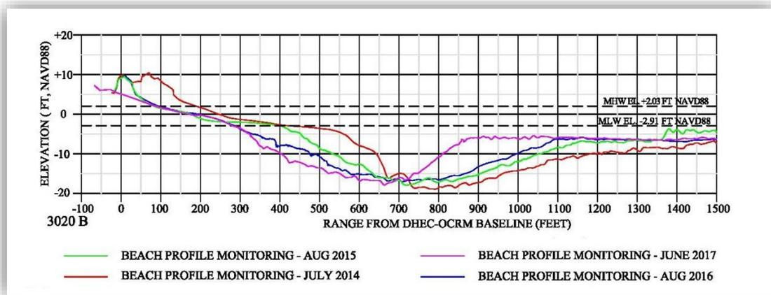
Figure 10. Beach profile monitoring data from 2014-2017 in cross-section view at Monument 3020.
