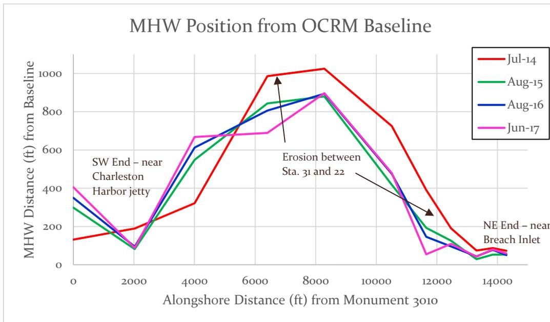
Figure 5. Annotated MHW Position graph illustrating the change in shoreline position from 2014 to 2017, as well as the distance between the shoreline and baseline.
