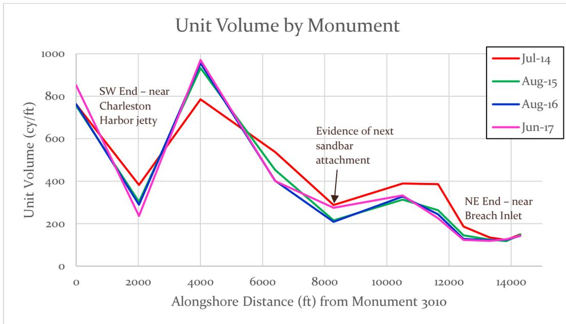
Figure 6. Annotated Unit Volume graph illustrating the change in unit volume at each profile from 2014 to 2017.
