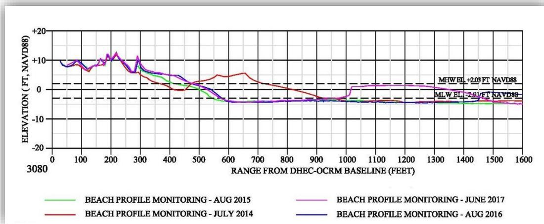
Figure 22. Beach profile monitoring data from 2014-2017 in cross-section view at Monument 3080.
