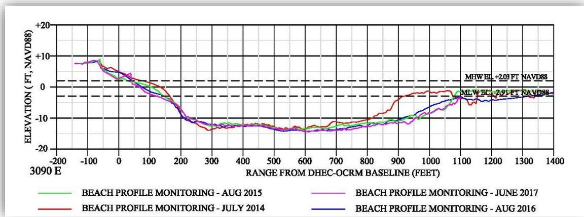
Figure 31. Beach profile monitoring data from 2014-2017 in cross-section view at Monument 3090.
