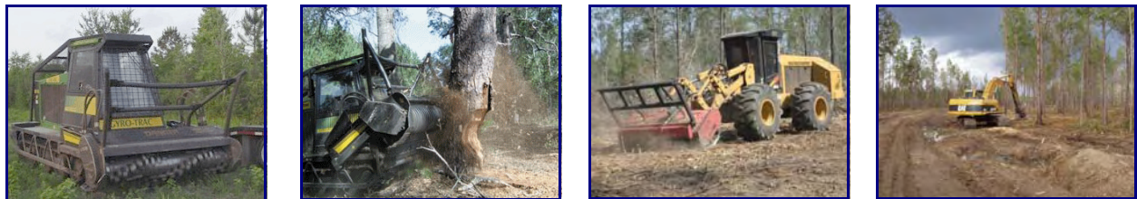
FIGURE 7.6. Mechanical equipment such as Gyro-Tracs®, Hydro-axes, and similar equipment would facilitate clearing of unwanted vegetation in the AL at possibly lower cost, but they are noisy and invasive.
