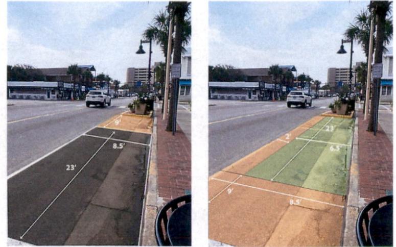
Example from City of Folly Beach Center Street Drainage Improvement. Siting of street level rain gardens
