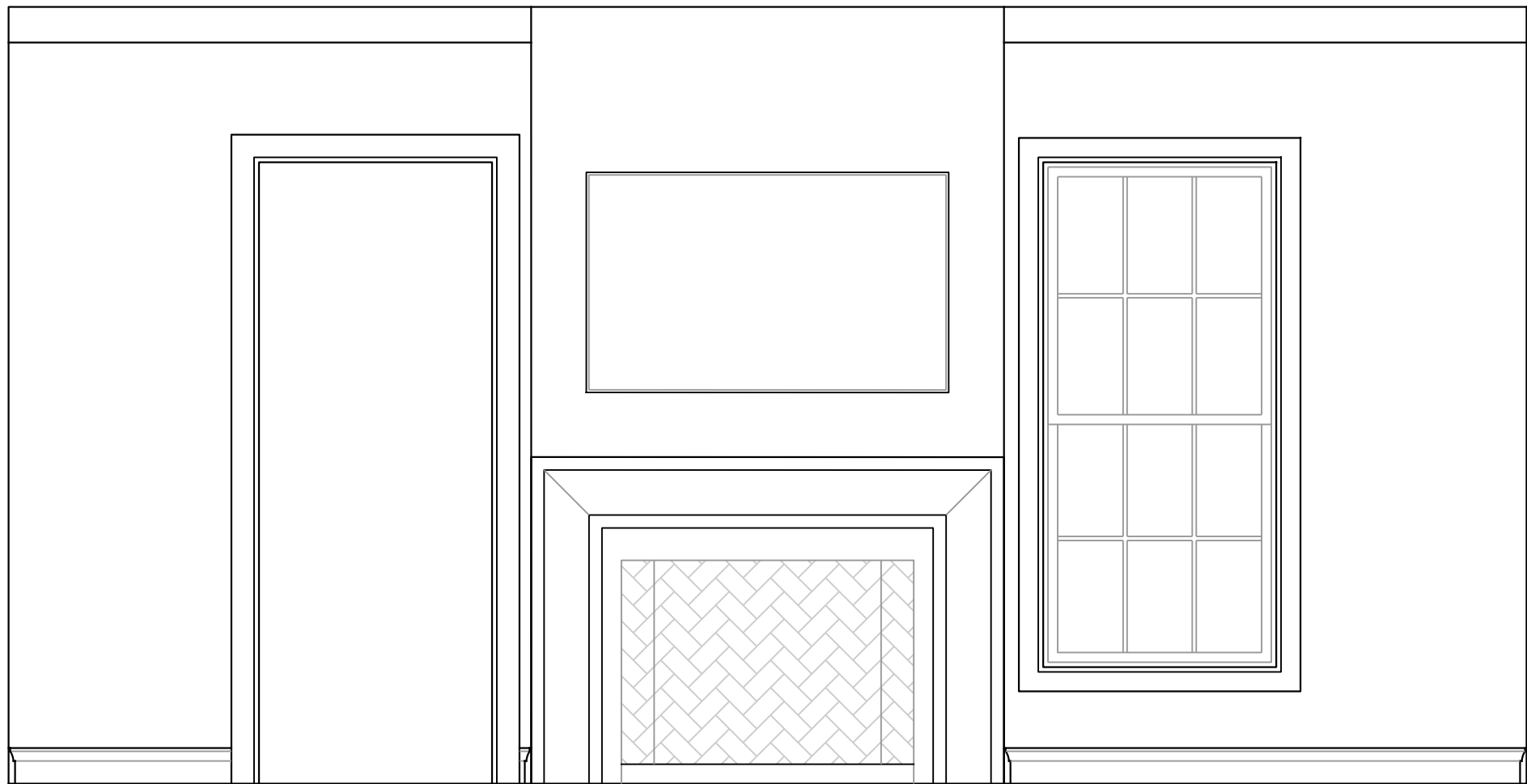
2 INTERIOR ELEVATION LIVING ROOM SCALE: 1/2"=1'-0"
