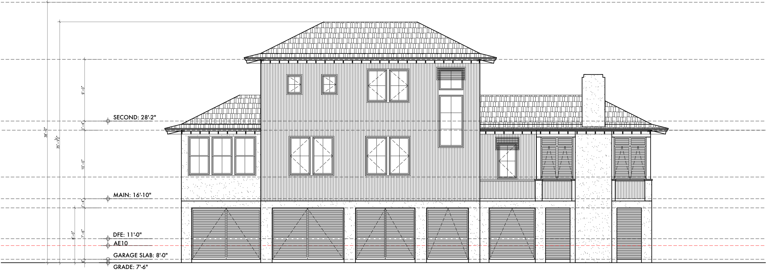
1 SOUTHWEST ELEVATION - PROPOSED scale 1/8"=1'-0"
