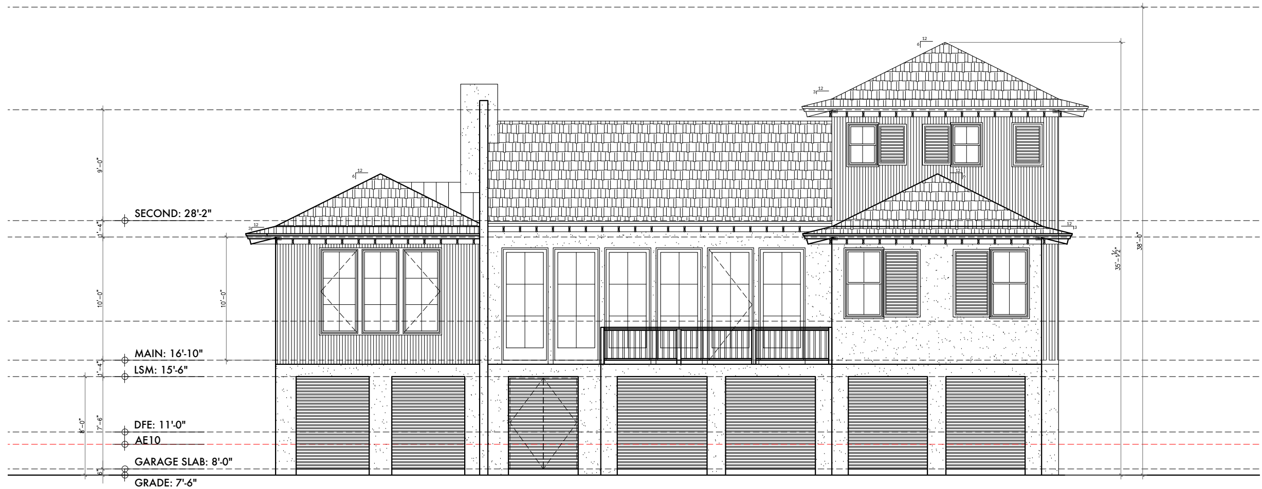
1 NORTHWEST ELEVATION - PROPOSED scale 1/8"=1'-0"
