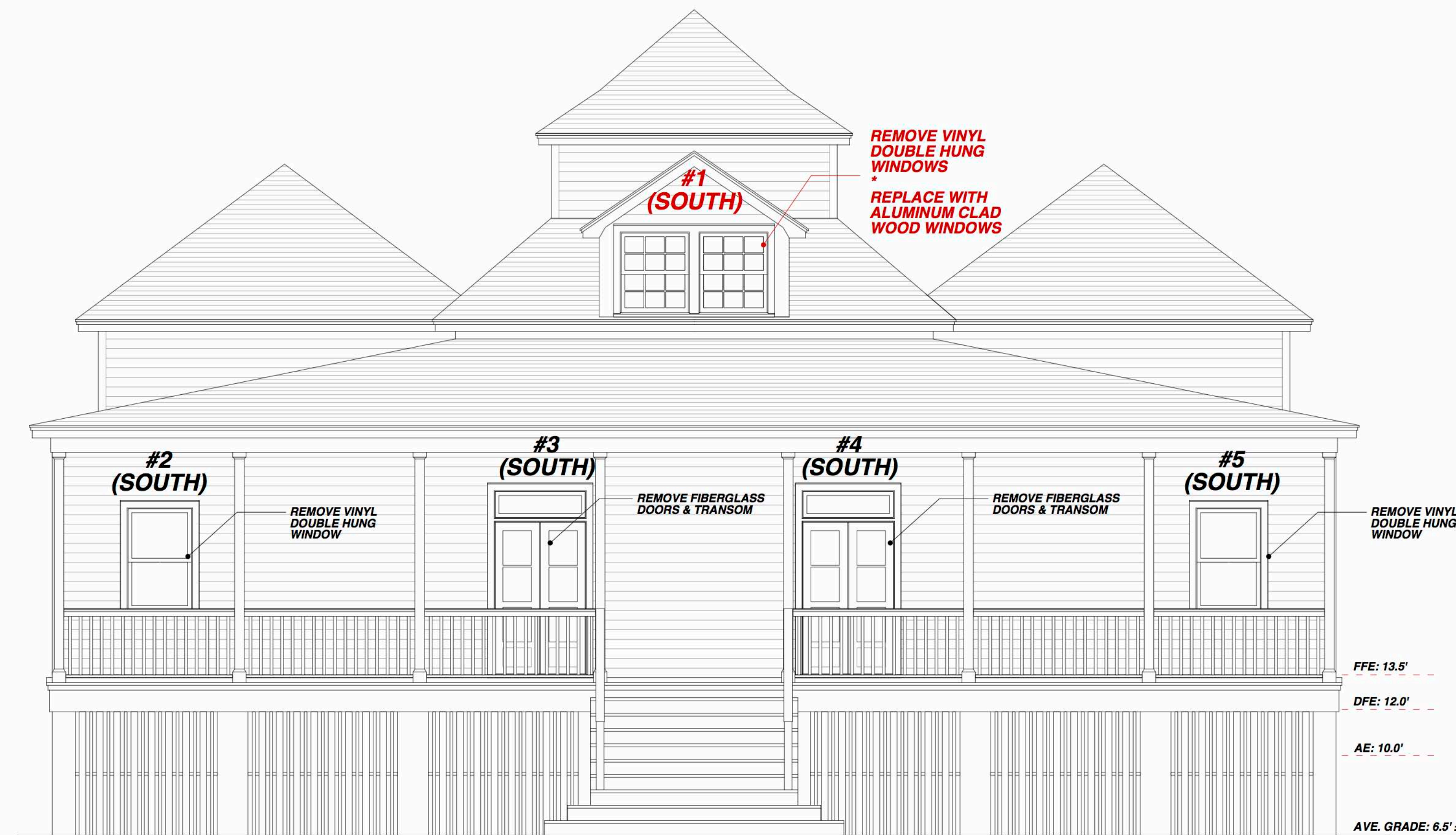
EXISTING: SOUTH (ION AVENUE) ELEVATION
