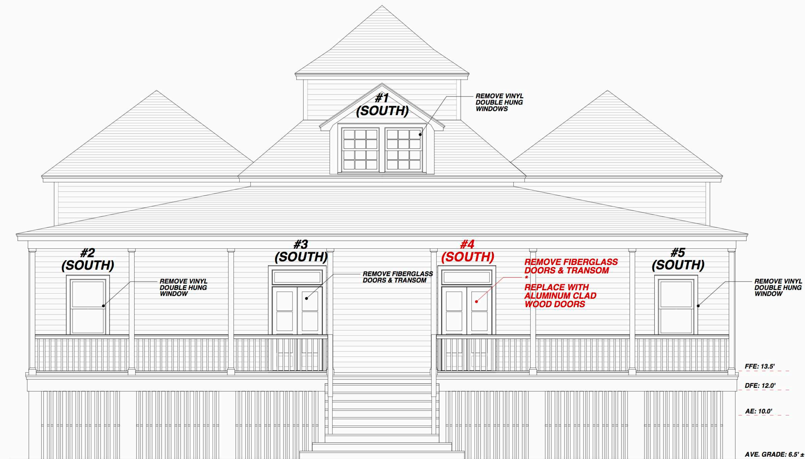
EXISTING: SOUTH (ION AVENUE) ELEVATION
