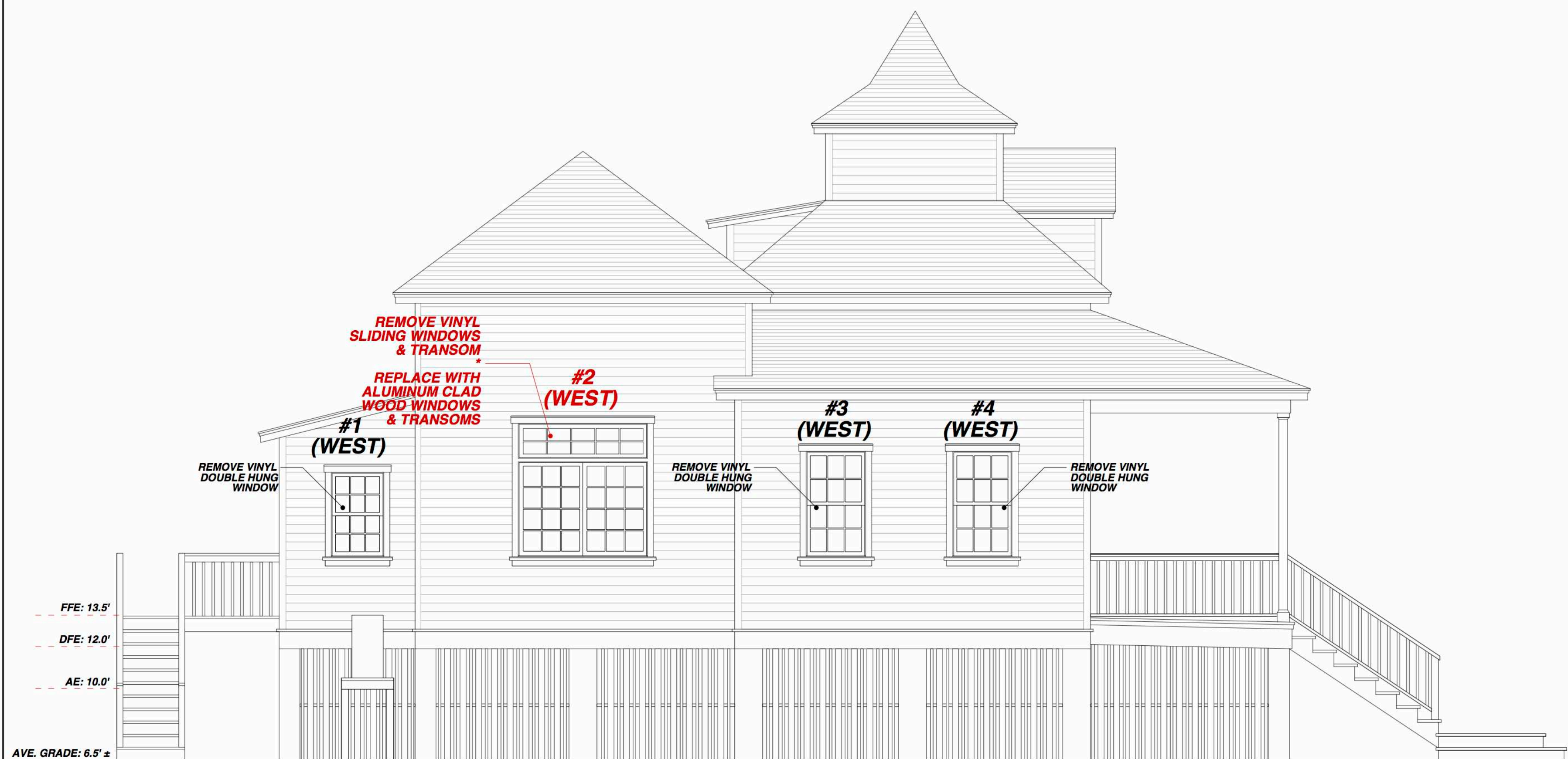
EXISTING: WEST (POOL SIDE) ELEVATION
