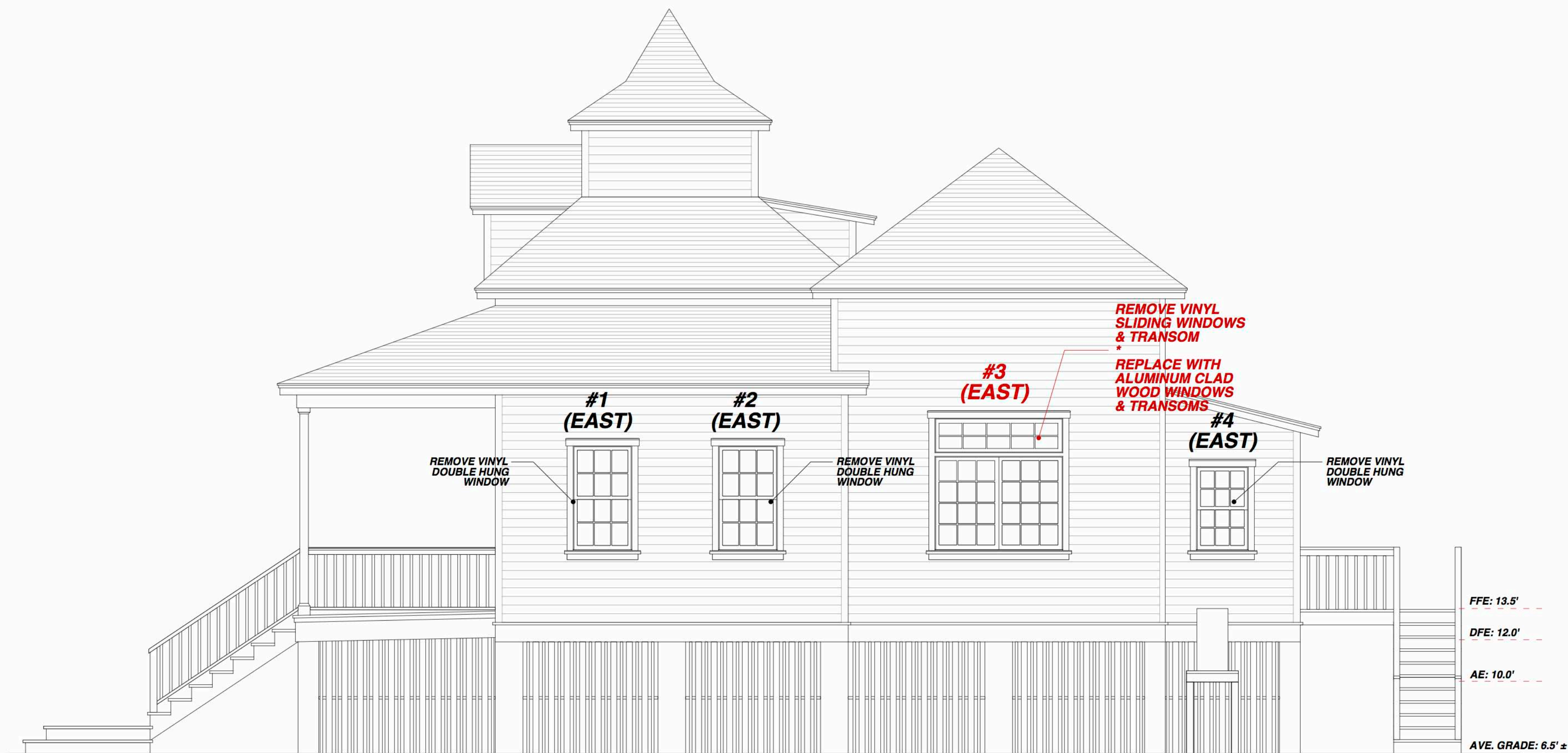
EXISTING: EAST (STATION 22 STREET) ELEVATION
