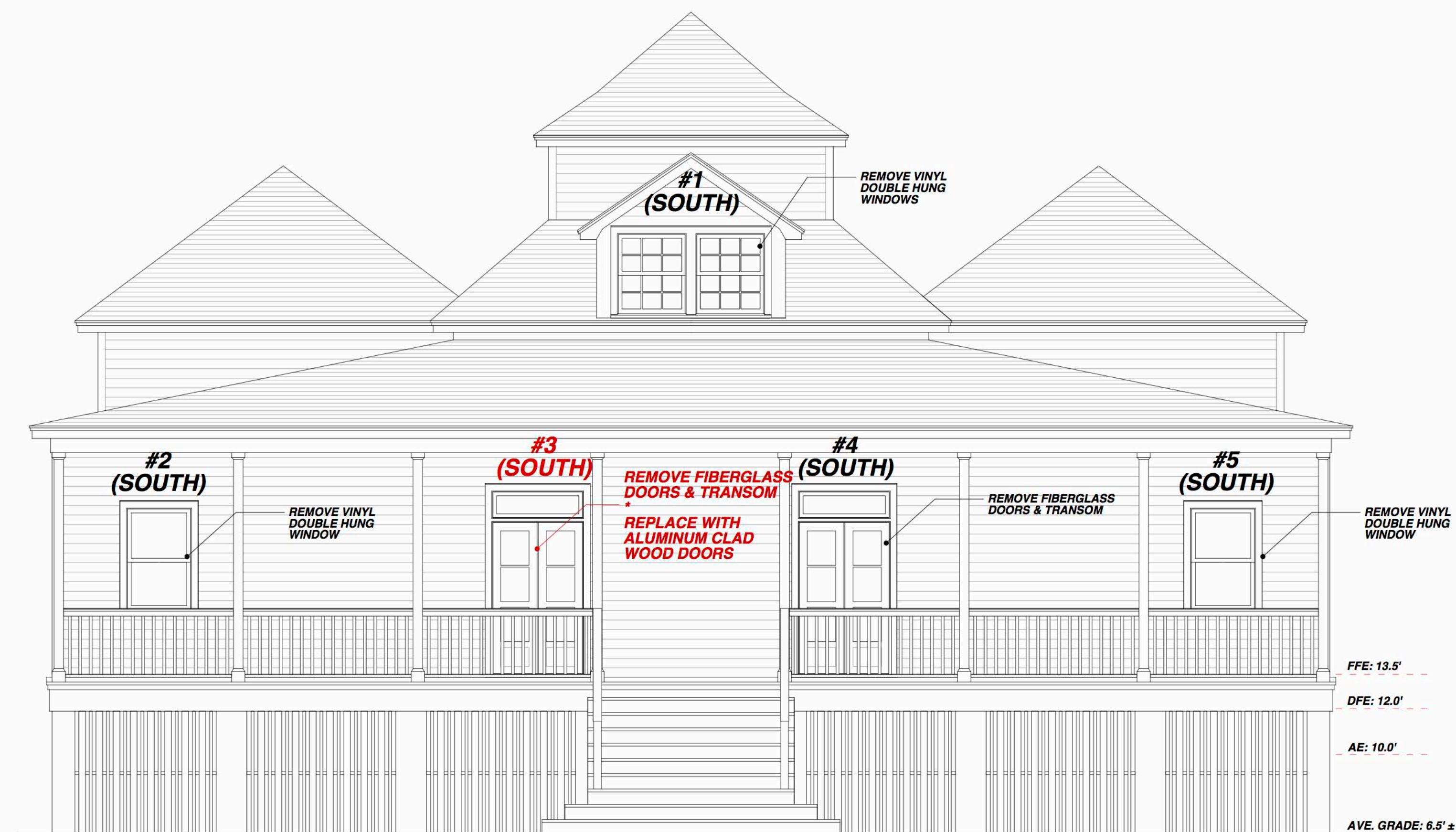
EXISTING: SOUTH (ION AVENUE) ELEVATION
