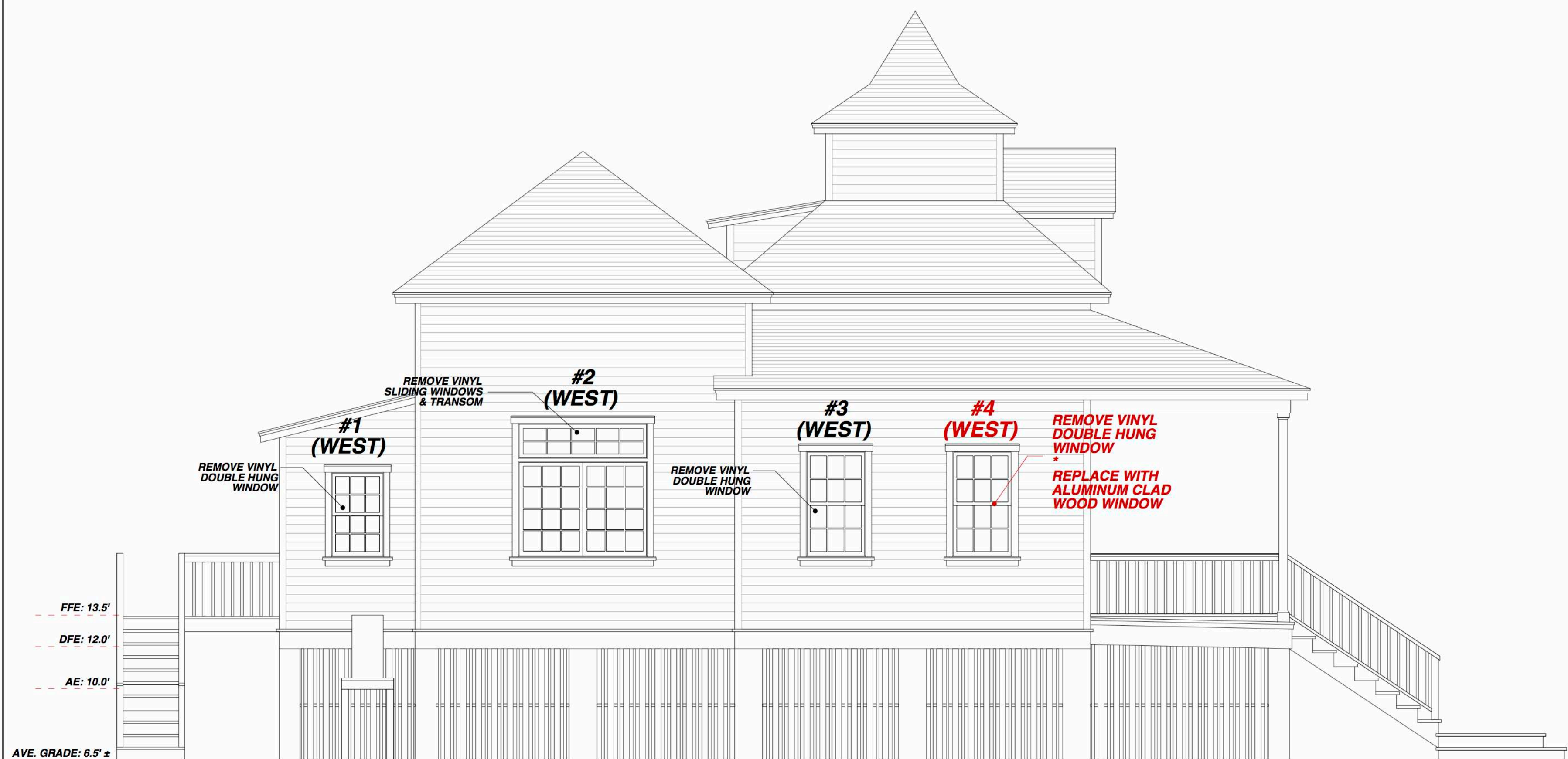
EXISTING: WEST (POOL SIDE) ELEVATION
