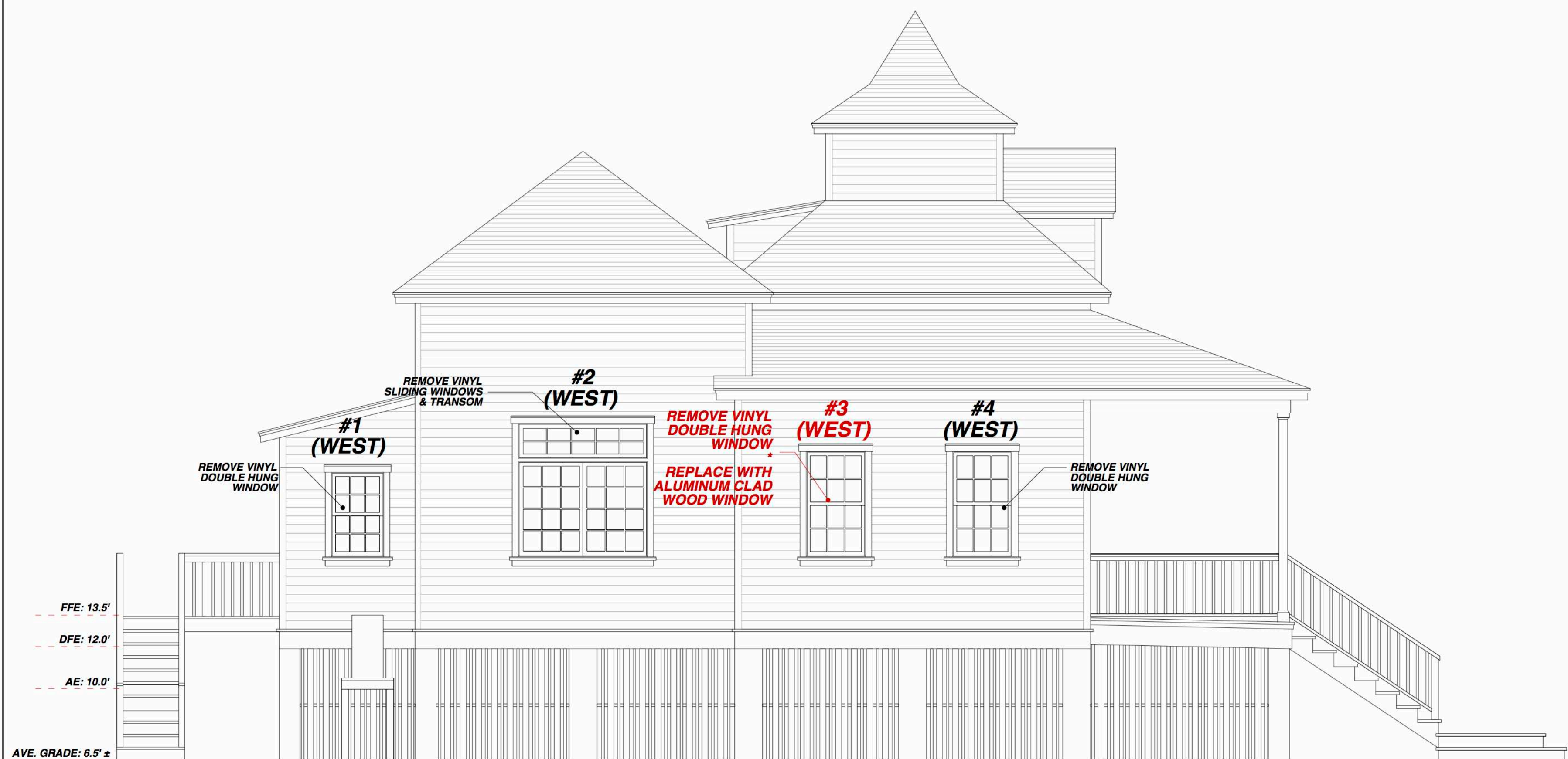
EXISTING: WEST (POOL SIDE) ELEVATION
