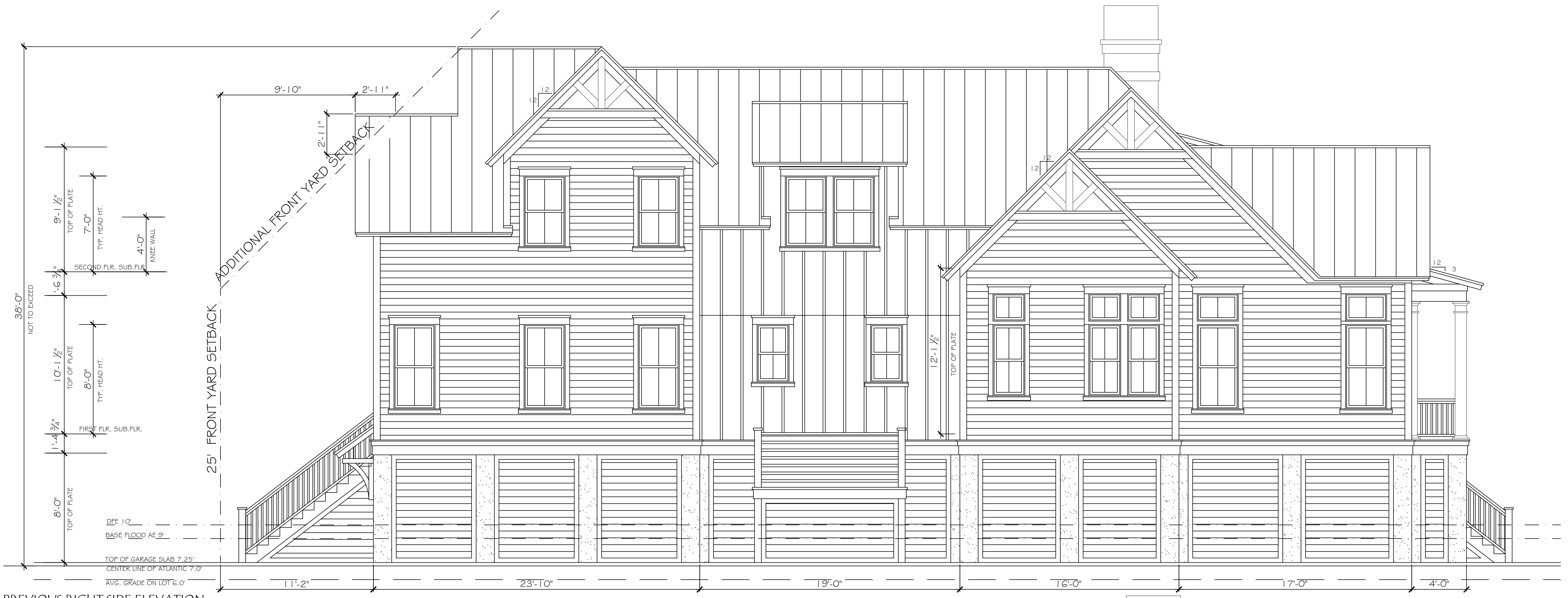
1 PREVIOUS RIGHT SIDE ELEVATION SCALE: 1/4" = 1'-0"
