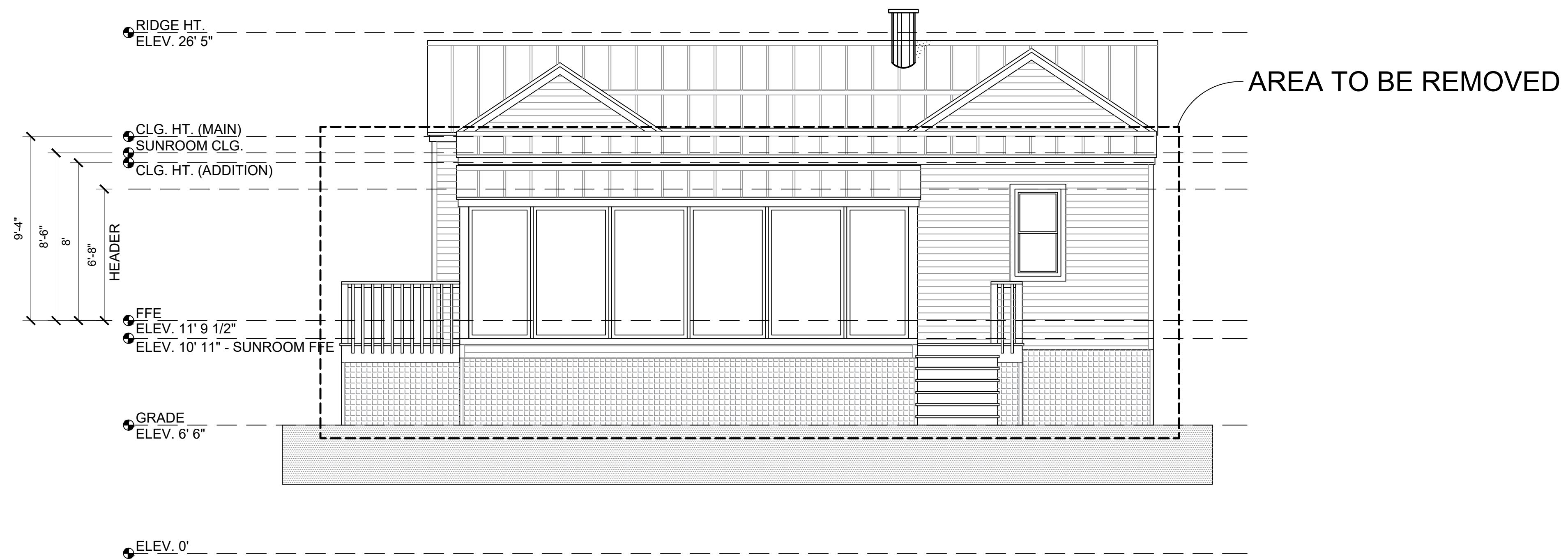
REAR ELEVATION - EXISTING 1/8" = 1'-0"
