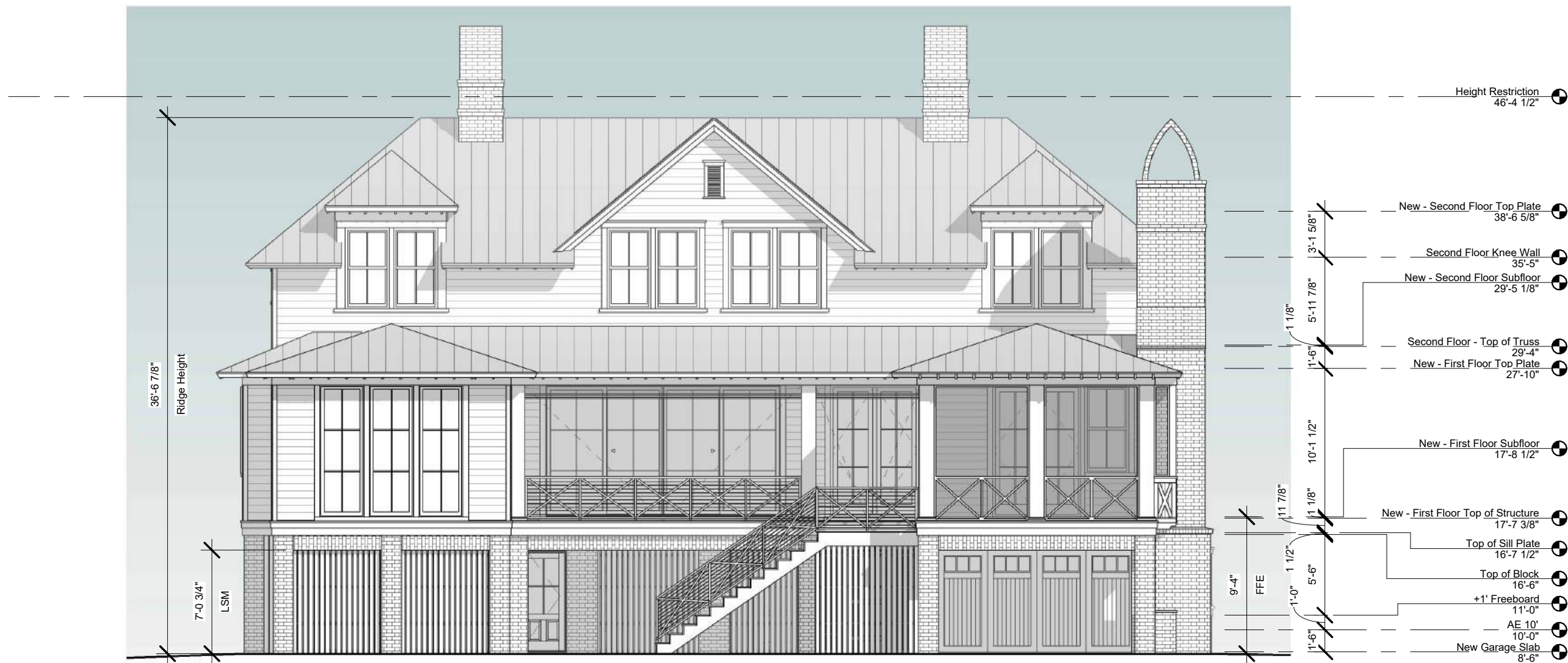
1 A2.4 Front Elevation - South - Main House 1/8" = 1'-0"
