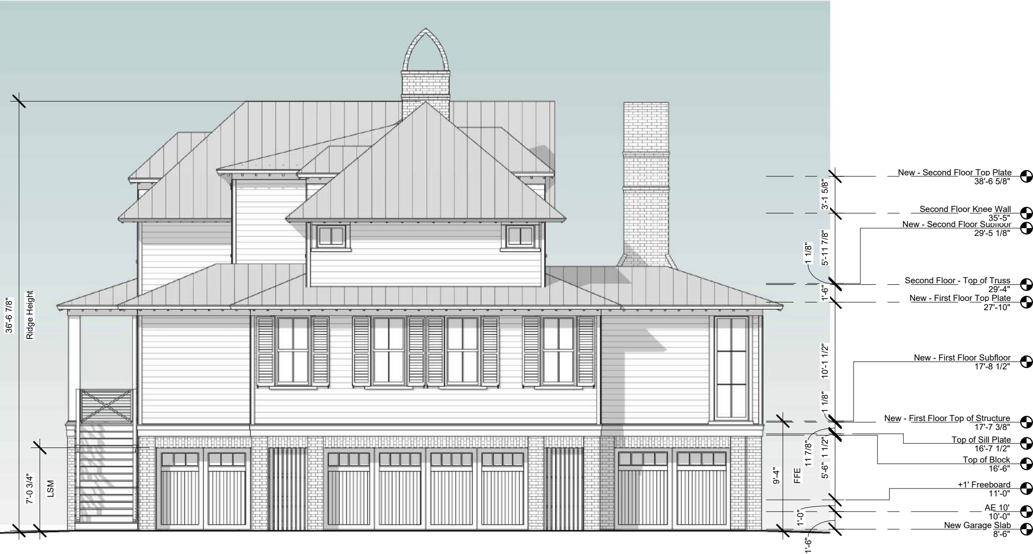
1 A2.6 Left Elevation - West - Proposed 1/8" = 1'-0"
