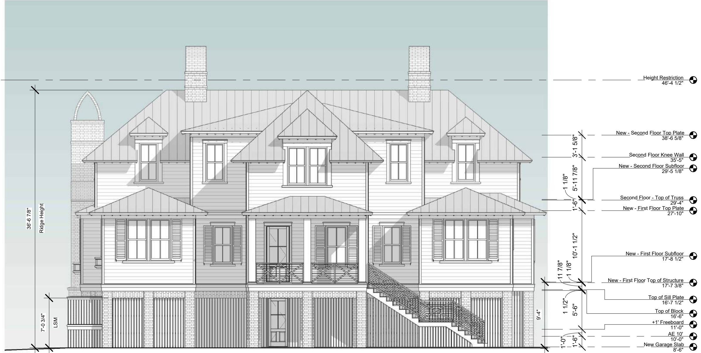
1 A2.5 Rear Elevation - North - Proposed 1/8" = 1'-0"
