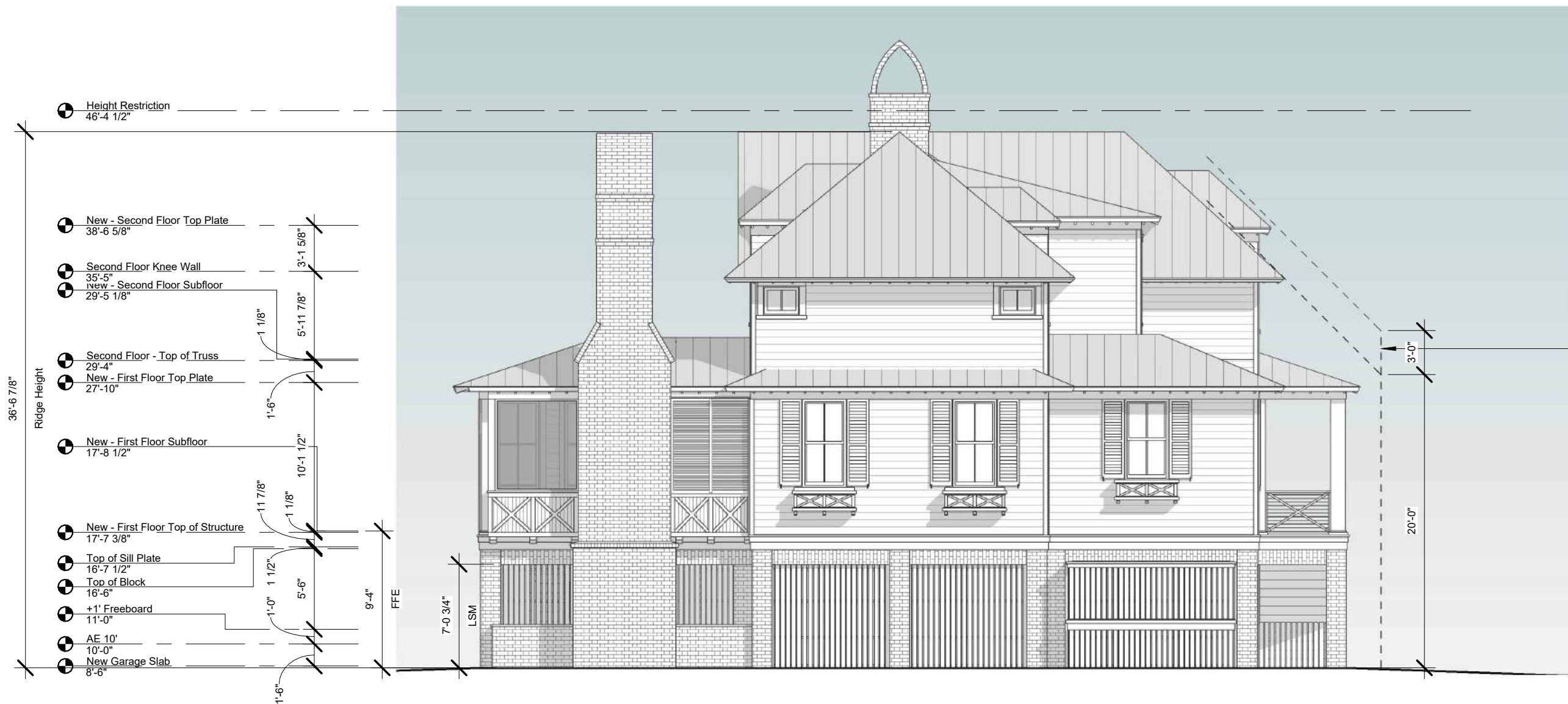
1 A2.7 Right Elevation - East - Proposed 1/8" = 1'-0"
