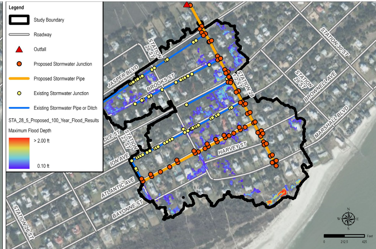
Existing (left) and proposed (right) flood results for the current conditions 100-Year (10.40”) and mean tide (static; -0.35’ NAVD88) scenario. Flood results assume all SCIP improvements have been implemented.
