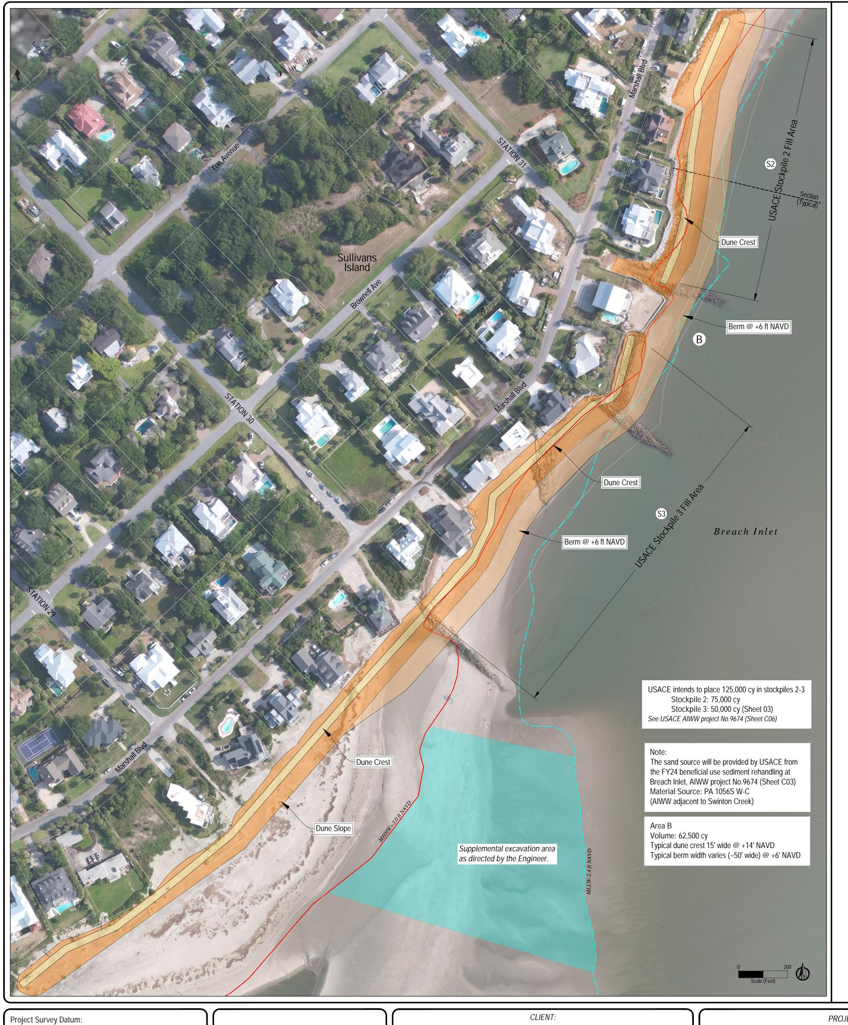
The sand source will be provided by USACE from the FY24 beneficial use sediment rehandling at Breach Inlet, AIWW project No.9674 (Sheet C03)
