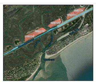
sediment will be excavated from the placement areas and transported hydraulically via dredge to the beaches adjacent to Breach Inlet on Isle of Palms and Sullivans Island. The project is funded in part by the Bi-partisan Infrastructure Law (BIL) as well as regular AIWW O&M Funding.
