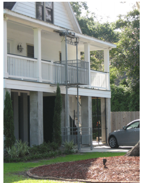
For high increase elevation buildings, chair lifts should be placed on rear or side elevations where they are less visible. This design has minimal structural framework and the porch can be viewed behind it.
