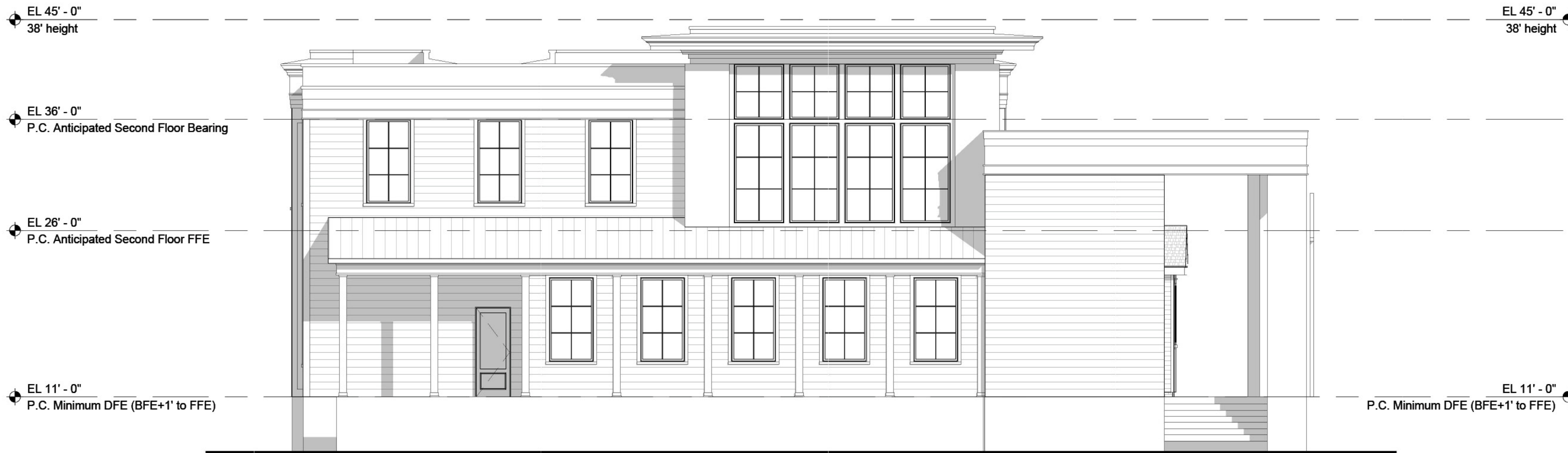
3 A202 Prop. Rear Elevation . NORTH SCALE: 1/8" = 1'-0"
