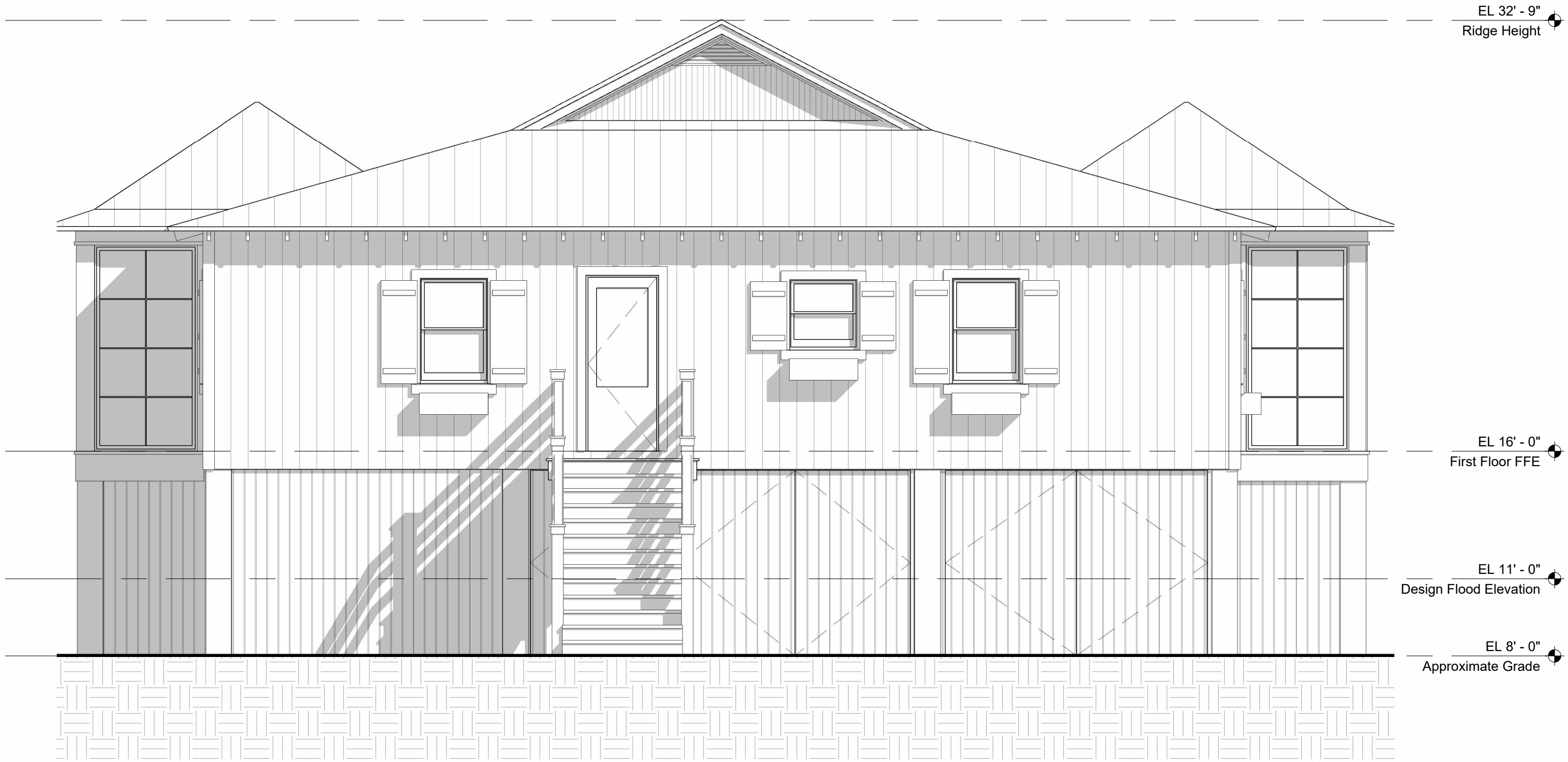
2 Proposed Front Elevation . NORTH SCALE: 1/4" = 1'-0"
