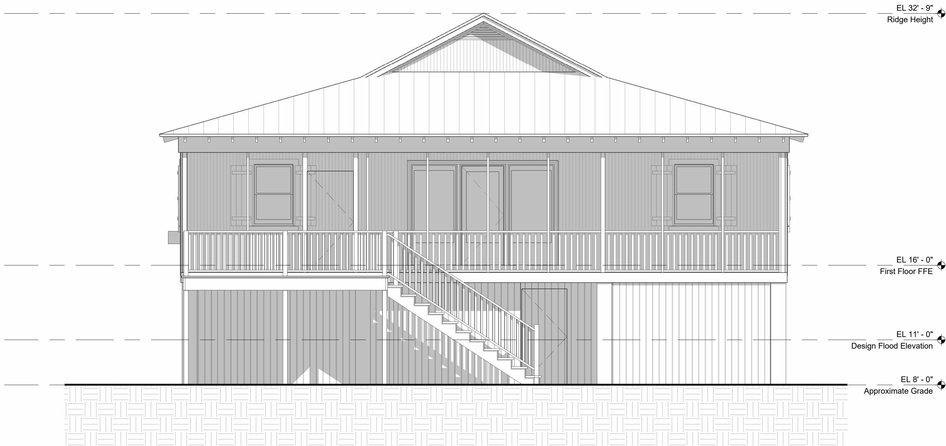
3 Existing Rear Elevation . SOUTH SCALE: 1/4" = 1'-0"
