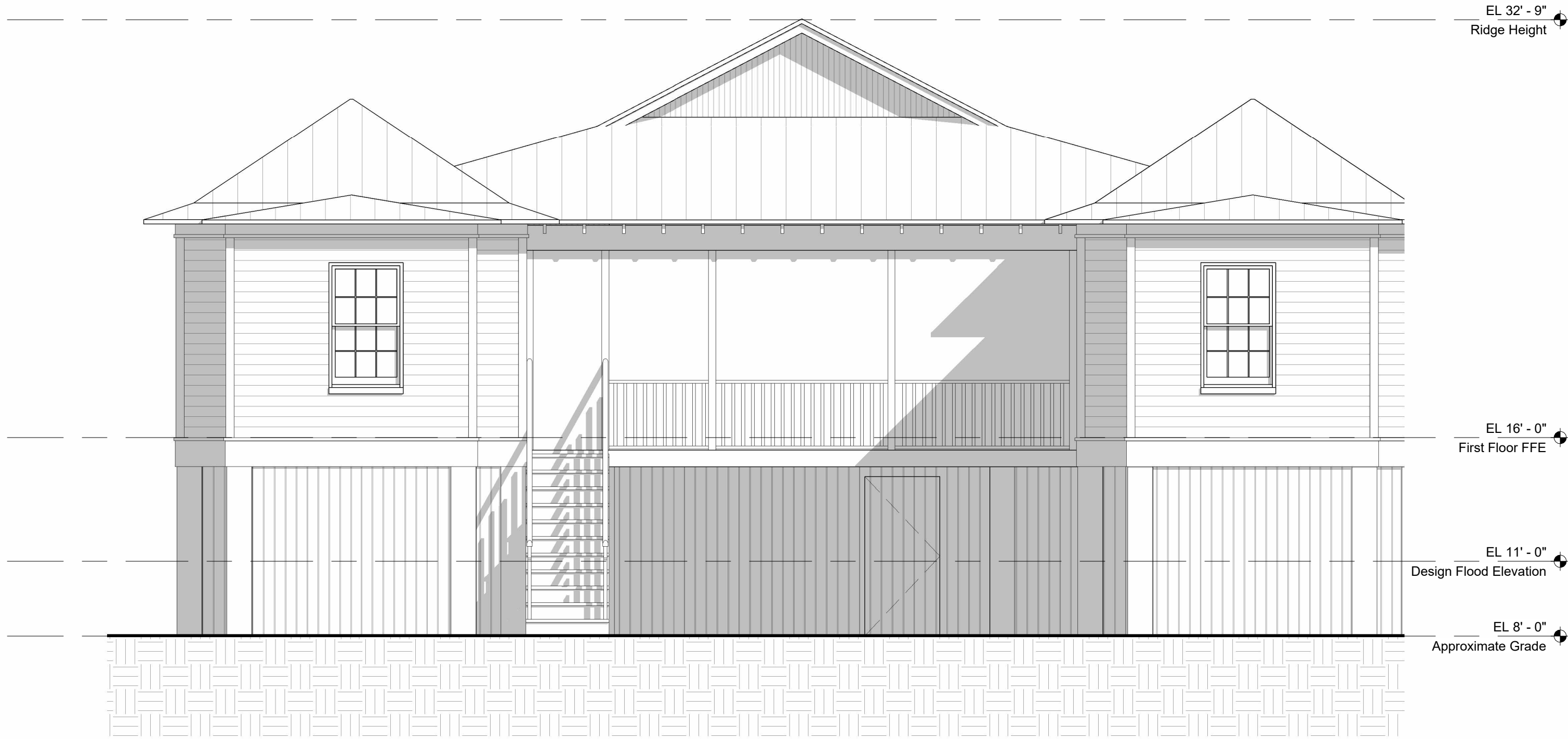
4 Proposed Rear Elevation . SOUTH SCALE: 1/4" = 1'-0"
