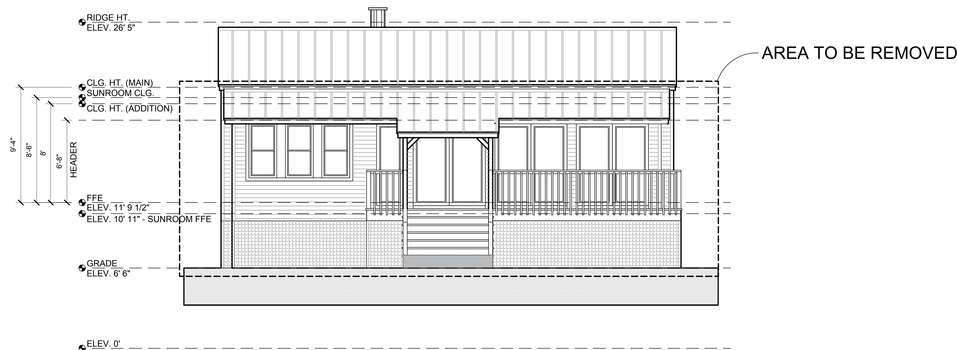
FRONT ELEVATION - EXISTING 1/8" = 1'-0"
